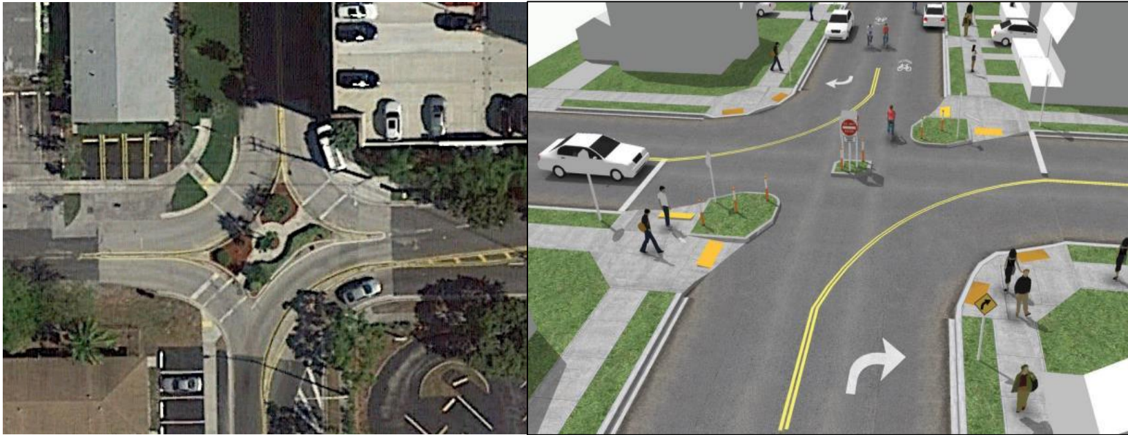
A Diagonal/Semi Diverters
