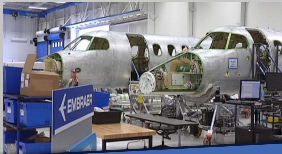
Executive jet airframes under construction at Embraer's manufacturing plant in Melbourne, FL.
