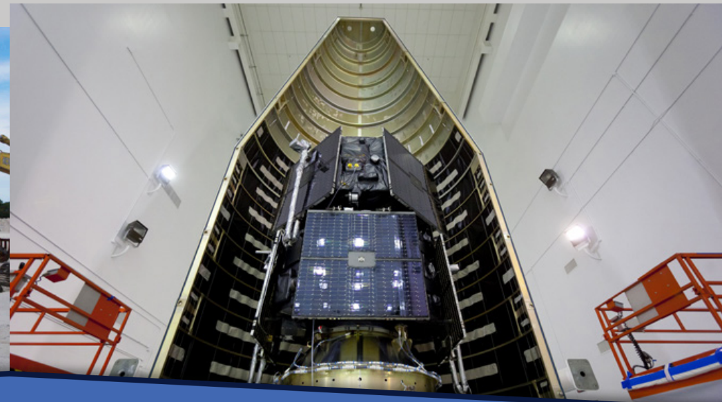
A satellite is placed into its cargo fairing at the former Astrotech Facility in Titusville.
