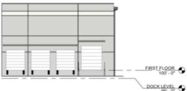
5 EXTERIOR ELEVATION - DOCK WALL - COLOR AS.3.1/ 1/16" = 1'-0"
