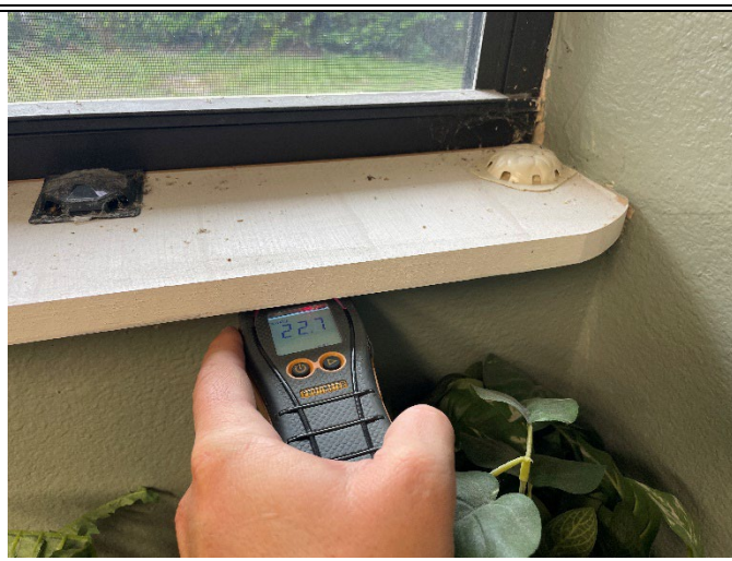
Photo 54: Elevated moisture was detected in the drywall below the break room window and rear wall.
