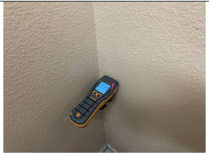
Photo 58: Elevated moisture was detected in the drywall on the left wall (near front corner) in the electrical room.
