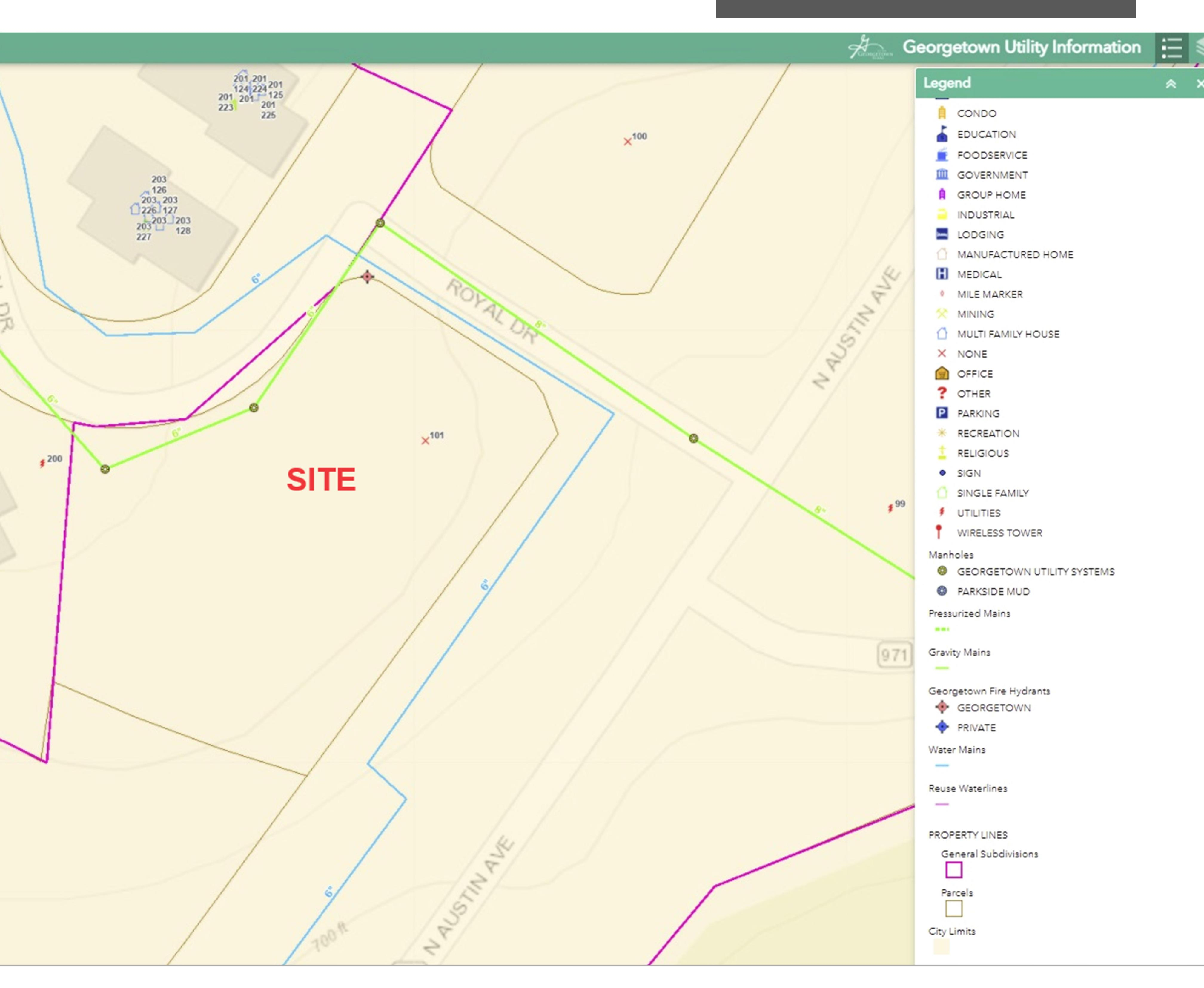
6" Water Line 6" Wastewater Line Electric to Site
