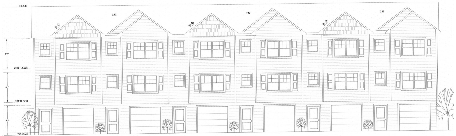
FRONT ELEVATION, BUILDING A (GARAGE BUILDING)
